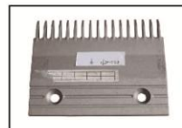
A-FLY ID: AF-HI20359C Part ID: 22501789A Size: 142.8*112.3*17T Hole distance :90 Material: aluminum Color: Silver/natural
