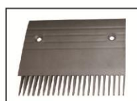
A-FLY ID: AF-FT140039A Part ID:FPA0104 Size: 199.5*154.3*2T Hole distance : 145 Material: aluminum Color: Silver/natural
