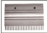
A-FLY ID: AF-OT80510A Part ID: GAA453BM1 Size: 203*139.2*24T Hole distance : 101.7 Material: aluminum Color: Silver/natural
