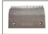
A-FLY ID: AF-OT80511B Part ID: HA453S2 Size: 203*133*22T Hole distance : 145 Material: aluminum Color: Silver/natural
