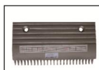
A-FLY ID: AF-OT80742C Part ID: XAA453AB8 Size: 214.2*111.2*25T Hole distance : 142.8 Material: aluminum Color: Silver/natural
