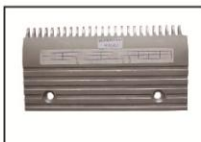
A-FLY ID: AF-OT80742B Part ID: XAA453AB7 Size: 214.2*111.2*25T Hole distance : 142.8 Material: aluminum Color: Silver/natural
