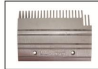
A-FLY ID: AF-OT80510E Part ID: GAA453BM7 Size: 198*139.2*23T Hole distance : 101.7 Material: aluminum Color: Silver/natural
