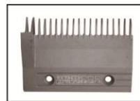
A-FLY ID: AF-HI20359A Part ID: 22501787A Size: 164.3*112.3*19T Hole distance :90 Material: aluminum Color: Silver/natural
